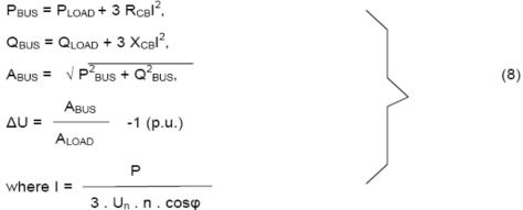
and  $R_{CB}$ ,  $X_{CB}$  are the cable parameters (R calculated at conductor's rated operating temperature).
