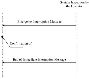
5. The Emergency Interruption Procedure at an NNGTS Entry Point/Reverse Flow Entry Point is summarised in the figure below:
