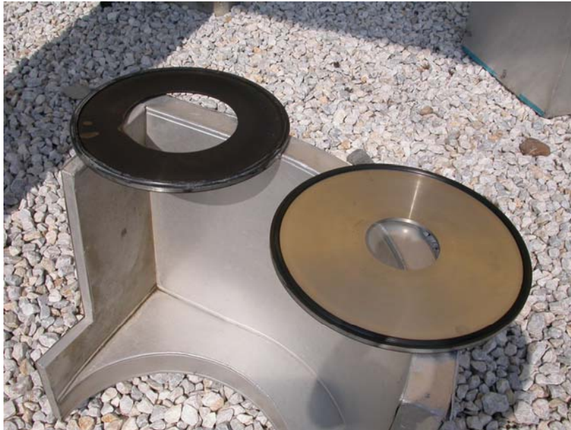
Figure 1. A contaminated with black powder ( left ) versus a clean ( right ) orifice plate. The bore diameter of the two orifice plates is different.
