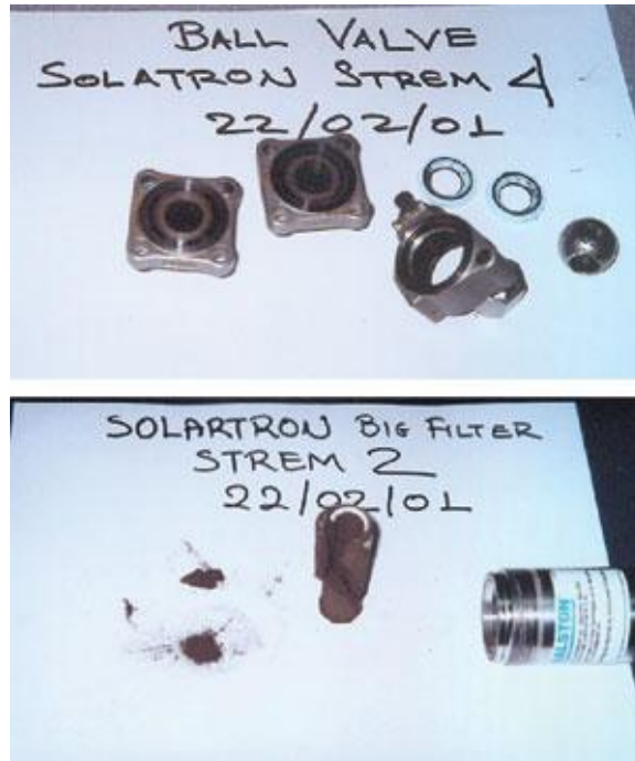
The photograph on the left shows parts of a ball valve from the feed line of an online densitometer heavily contaminated by black powder. The right photograph shows the inlet filter element of a similarly contaminated online densitometer (Fig.6).
